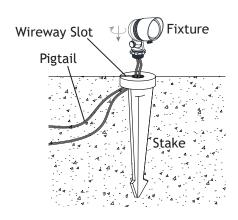
Clear away an area in the ground at the wireway slot on top of the stake. Lay the luminaire pigtail into the wireway slot and screw the fixture on to the stake. Tighten until snug.
