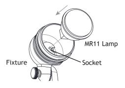
Insert the MR11 lamp with correct wattage and type marked on fixture label.
