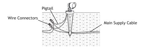
Strip both the leads from the luminaire pigtail. Using two UL listed wire connectors (sold separately), connect the leads from the luminaire to the main supply cable leads.
