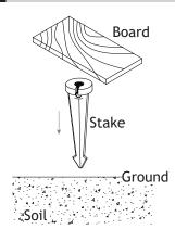
Determine the desired location for mounting the fixture. Hammer the stake into the ground until flange of stake is flush to grade. To avoid damage to the stake, place a board on top of the stake while hammering.
