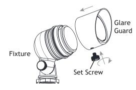
Place the glare guard back onto the fixture and secure with previously removed set screw.
