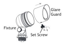
Loosen the set screw and remove the glare guard from the fixture.
